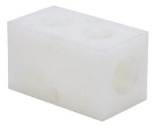
NITRA pneumatic or water valve manifold, Nylon 6, white, rectangular, 200 psi maximum operating pressure, (2) stations, (2) 1/4in female NPT inlet(s), (2) 1/8in female NPT outlet(s), standard hole spacing.
