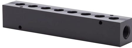
NITRA pneumatic valve manifold, aluminum, black, rectangular, 1000 psi maximum operating pressure, (8) stations, (2) 1/2in female NPT inlet(s), (8) 3/8in female NPT outlet(s), standard hole spacing.
