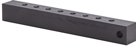
NITRA pneumatic valve manifold, aluminum, black, rectangular, 1000 psi maximum operating pressure, (8) stations, (1) 1/8in female NPT inlet(s), (16) #10-32 female UNF outlet(s), 180-degree orientation, standard hole spacing.
