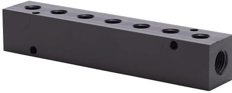
NITRA pneumatic valve manifold, aluminum, black, rectangular, 1000 psi maximum operating pressure, (7) stations, (2) 1/4in female NPT inlet(s), (7) 1/8in female NPT outlet(s), standard hole spacing.
