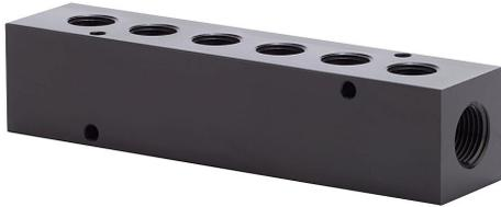
NITRA pneumatic valve manifold, aluminum, black, rectangular, 1000 psi maximum operating pressure, (6) stations, (2) 1/2in female NPT inlet(s), (6) 3/8in female NPT outlet(s), standard hole spacing.
