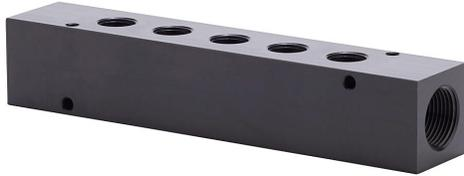
NITRA pneumatic valve manifold, aluminum, black, rectangular, 1000 psi maximum operating pressure, (5) stations, (2) 3/4in female NPT inlet(s), (5) 3/8in female NPT outlet(s), standard hole spacing.
