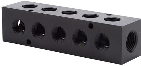
NITRA pneumatic valve manifold, aluminum, black, rectangular, 1000 psi maximum operating pressure, (5) stations, (2) 1/2in female NPT inlet(s), (10) 3/8in female NPT outlet(s), 90-degree orientation, standard hole spacing.
