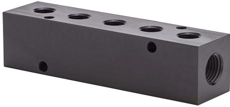
NITRA pneumatic valve manifold, aluminum, black, rectangular, 1000 psi maximum operating pressure, (5) stations, (2) 1/4in female NPT inlet(s), (5) 1/8in female NPT outlet(s), standard hole spacing.
