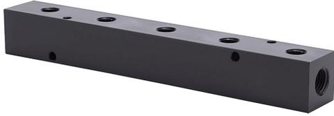
NITRA pneumatic valve manifold, aluminum, black, rectangular, 1000 psi maximum operating pressure, (5) stations, (2) 1/4in female NPT inlet(s), (5) 1/8in female NPT outlet(s), wide hole spacing.
