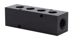
NITRA pneumatic valve manifold, aluminum, black, rectangular, 1000 psi maximum operating pressure, (4) stations, (2) 1/2in female NPT inlet(s), (4) 3/8in female NPT outlet(s), standard hole spacing.
