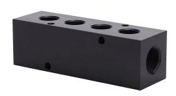
NITRA pneumatic valve manifold, aluminum, rectangular, 1000 psi maximum operating pressure, (4) stations, (2) 1/2in female NPT inlet(s), (4) 3/8in female NPT outlet(s), standard hole spacing.
