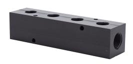
NITRA pneumatic valve manifold, aluminum, black, rectangular, 1000 psi maximum operating pressure, (4) stations, (2) 1/2in female NPT inlet(s), (4) 3/8in female NPT outlet(s), wide hole spacing.
