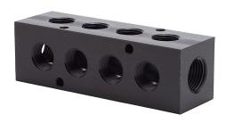
NITRA pneumatic valve manifold, aluminum, black, rectangular, 1000 psi maximum operating pressure, (4) stations, (2) 1/2in female NPT inlet(s), (8) 3/8in female NPT outlet(s), 90-degree orientation, standard hole spacing.
