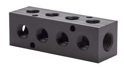
NITRA pneumatic valve manifold, aluminum, black, rectangular, 1000 psi maximum operating pressure, (4) stations, (2) 3/8in female NPT inlet(s), (8) 1/4in female NPT outlet(s), 90-degree orientation, standard hole spacing.
