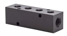
NITRA pneumatic valve manifold, aluminum, black, rectangular, 1000 psi maximum operating pressure, (4) stations, (2) 1/4in female NPT inlet(s), (4) 1/8in female NPT outlet(s), standard hole spacing.
