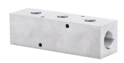
NITRA pneumatic valve manifold, aluminum, rectangular, 1000 psi maximum operating pressure, (3) stations, (2) 1in female NPT inlet(s), (3) 1/2in female NPT outlet(s), standard hole spacing.
