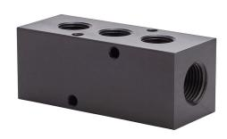
NITRA pneumatic valve manifold, aluminum, black, rectangular, 1000 psi maximum operating pressure, (3) stations, (2) 1/2in female NPT inlet(s), (3) 3/8in female NPT outlet(s), standard hole spacing.
