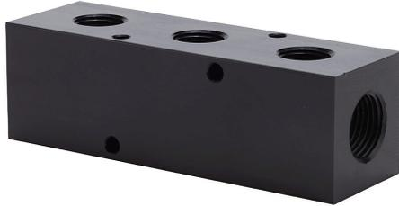
NITRA pneumatic valve manifold, aluminum, black, rectangular, 1000 psi maximum operating pressure, (3) stations, (2) 1/2in female NPT inlet(s), (3) 3/8in female NPT outlet(s), wide hole spacing.
