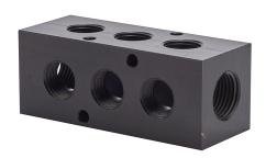
NITRA pneumatic valve manifold, aluminum, rectangular, 1000 psi maximum operating pressure, (3) stations, (2) 1/2in female NPT inlet(s), (6) 3/8in female NPT outlet(s), 90-degree orientation, standard hole spacing.
