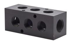
NITRA pneumatic valve manifold, aluminum, black, rectangular, 1000 psi maximum operating pressure, (3) stations, (2) 1/2in female NPT inlet(s), (6) 3/8in female NPT outlet(s), 90-degree orientation, standard hole spacing.
