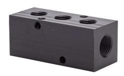
NITRA pneumatic valve manifold, aluminum, black, rectangular, 1000 psi maximum operating pressure, (3) stations, (2) 3/8in female NPT inlet(s), (3) 1/4in female NPT outlet(s), standard hole spacing.
