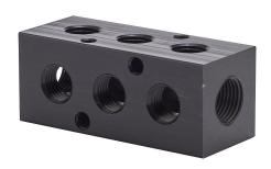
NITRA pneumatic valve manifold, aluminum, black, rectangular, 1000 psi maximum operating pressure, (3) stations, (2) 3/8in female NPT inlet(s), (6) 1/4in female NPT outlet(s), 90-degree orientation, standard hole spacing.
