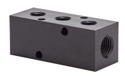
NITRA pneumatic valve manifold, aluminum, rectangular, 1000 psi maximum operating pressure, (3) stations, (2) 1/4in female NPT inlet(s), (3) 1/8in female NPT outlet(s), standard hole spacing.
