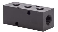
NITRA pneumatic valve manifold, aluminum, black, rectangular, 1000 psi maximum operating pressure, (3) stations, (2) 1/4in female NPT inlet(s), (3) 1/8in female NPT outlet(s), standard hole spacing.
