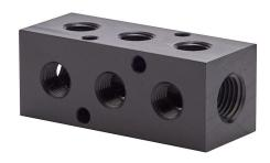
NITRA pneumatic valve manifold, aluminum, black, rectangular, 1000 psi maximum operating pressure, (3) stations, (2) 1/4in female NPT inlet(s), (6) 1/8in female NPT outlet(s), 90-degree orientation, standard hole spacing.
