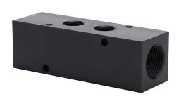
NITRA pneumatic valve manifold, aluminum, black, rectangular, 1000 psi maximum operating pressure, (2) stations, (2) 3/4in female NPT inlet(s), (2) 3/8in female NPT outlet(s), standard hole spacing.
