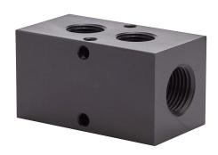
NITRA pneumatic valve manifold, aluminum, rectangular, 1000 psi maximum operating pressure, (2) stations, (2) 1/2in female NPT inlet(s), (2) 3/8in female NPT outlet(s), standard hole spacing.
