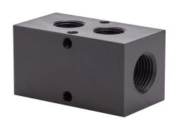
NITRA pneumatic valve manifold, aluminum, black, rectangular, 1000 psi maximum operating pressure, (2) stations, (2) 1/2in female NPT inlet(s), (2) 3/8in female NPT outlet(s), standard hole spacing.
