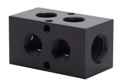
NITRA pneumatic valve manifold, aluminum, black, rectangular, 1000 psi maximum operating pressure, (2) stations, (2) 1/2in female NPT inlet(s), (4) 3/8in female NPT outlet(s), 90-degree orientation, standard hole spacing.
