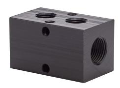
NITRA pneumatic valve manifold, aluminum, black, rectangular, 1000 psi maximum operating pressure, (2) stations, (2) 3/8in female NPT inlet(s), (2) 1/4in female NPT outlet(s), standard hole spacing.
