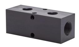
NITRA pneumatic valve manifold, aluminum, black, rectangular, 1000 psi maximum operating pressure, (2) stations, (2) 3/8in female NPT inlet(s), (2) 1/4in female NPT outlet(s), wide hole spacing.
