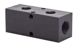
NITRA pneumatic valve manifold, aluminum, rectangular, 1000 psi maximum operating pressure, (2) stations, (2) 3/8in female NPT inlet(s), (2) 1/4in female NPT outlet(s), wide hole spacing.
