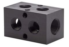
NITRA pneumatic valve manifold, aluminum, black, rectangular, 1000 psi maximum operating pressure, (2) stations, (2) 3/8in female NPT inlet(s), (4) 1/4in female NPT outlet(s), 90-degree orientation, standard hole spacing.
