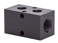
NITRA pneumatic valve manifold, aluminum, black, rectangular, 1000 psi maximum operating pressure, (2) stations, (2) 1/4in female NPT inlet(s), (2) 1/8in female NPT outlet(s), standard hole spacing.
