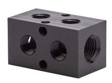
NITRA pneumatic valve manifold, aluminum, black, rectangular, 1000 psi maximum operating pressure, (2) stations, (2) 1/4in female NPT inlet(s), (4) 1/8in female NPT outlet(s), 90-degree orientation, standard hole spacing.
