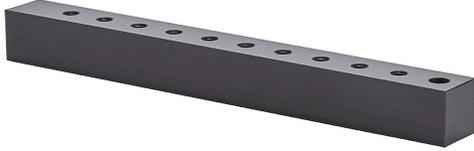
NITRA pneumatic valve manifold, aluminum, black, rectangular, 1000 psi maximum operating pressure, (10) stations, (1) 1/8in female NPT inlet(s), (10) #10-32 female UNF outlet(s), standard hole spacing.
