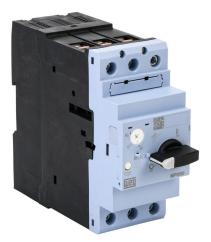
WEG Electric MPW80 series manual motor protector, rotary, 65A, thermal overload, 50.0-65.0A adjustable, 845A instantaneous trip rating, open, 54mm frame.
