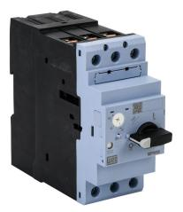
WEG Electric MPW80 series manual motor protector, rotary, 50A, thermal overload, 40.0-50.0A adjustable, 650A instantaneous trip rating, open, 54mm frame.
