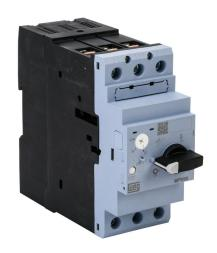
WEG Electric MPW80 series manual motor protector, rotary, 40A, thermal overload, 32.0-40.0A adjustable, 520A instantaneous trip rating, open, 54mm frame.
