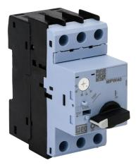
WEG Electric MPW40 series manual motor protector, rotary, 40A, thermal overload, 32.0-40.0A adjustable, 520A instantaneous trip rating, open, 45mm frame.
