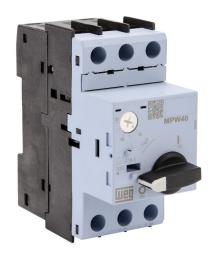
WEG Electric MPW40 series manual motor protector, rotary, 32A, thermal overload, 25.0-32.0A adjustable, 416A instantaneous trip rating, open, 45mm frame.
