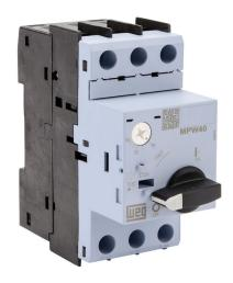
WEG Electric MPW40 series manual motor protector, rotary, 25A, thermal overload, 20.0-25.0A adjustable, 325A instantaneous trip rating, open, 45mm frame.
