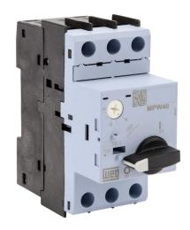
WEG Electric MPW40 series manual motor protector, rotary, 20A, thermal overload, 16.0-20.0A adjustable, 260A instantaneous trip rating, open, 45mm frame.
