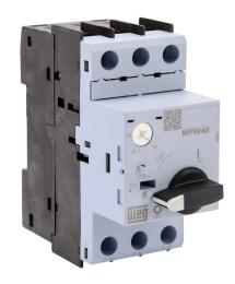
WEG Electric MPW40 series manual motor protector, rotary, 16A, thermal overload, 10.0-16.0A adjustable, 208A instantaneous trip rating, open, 45mm frame.
