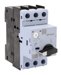
WEG Electric MPW40 series manual motor protector, rotary, 1A, thermal overload, 0.63-1.0A adjustable, 13A instantaneous trip rating, open, 45mm frame.
