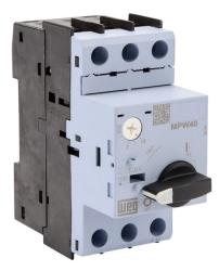
WEG Electric MPW40 series manual motor protector, rotary, 2.5A, thermal overload, 1.6-2.5A adjustable, 32.5A instantaneous trip rating, open, 45mm frame.
