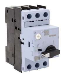
WEG Electric MPW40 series manual motor protector, rotary, 1.6A, thermal overload, 1.0-1.6A adjustable, 20.8A instantaneous trip rating, open, 45mm frame.
