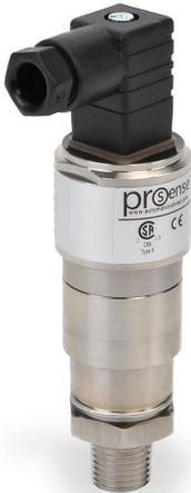
ProSense mechanical pressure switch, 50 to 500 psig set point, 316 stainless steel piston sensing element, Buna-N O-ring seal(s), SPDT 3A, 1/4in male NPT process connection, DIN 175301-803C L-connector.
