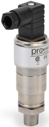
ProSense mechanical pressure switch, 40 to 200 psig set point, 316 stainless steel piston sensing element, Buna-N O-ring seal(s), SPDT 3A, 1/4in male NPT process connection, DIN 175301-803C L-connector.
