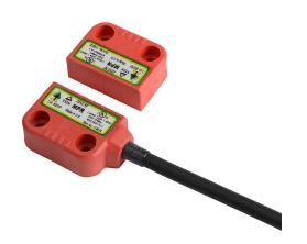
IDEM safety switch set, non-contact magnetic, left exit mount, (2) N.C. safety output(s), (1) N.O. monitoring output(s), plastic housing, 36 x 26mm, 8-pin M12 quick-disconnect, 9.8in/250mm cable length.
