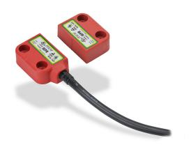
IDEM safety switch set, non-contact magnetic, left exit mount, (2) N.C. safety output(s), (1) N.O. monitoring output(s), plastic housing, 36 x 26mm, pigtail, 32.8ft/10m cable length.
