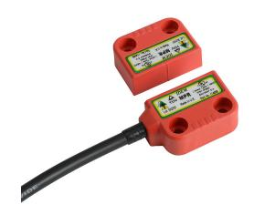
IDEM safety switch set, non-contact magnetic, right exit mount, (2) N.C. safety output(s), (1) N.O. monitoring output(s), plastic housing, 36 x 26mm, 8-pin M12 quick-disconnect, 9.8in/250mm cable length.
