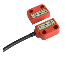
IDEM safety switch set, non-contact magnetic, right exit mount, (2) N.C. safety output(s), (1) N.O. monitoring output(s), plastic housing, 36 x 26mm, 8-pin M12 quick-disconnect, 9.8in/250mm cable length.
