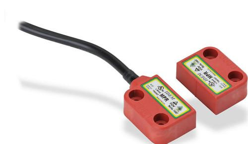
IDEM safety switch set, non-contact magnetic, right exit mount, (2) N.C. safety output(s), (1) N.O. monitoring output(s), plastic housing, 36 x 26mm, pigtail, 32.8ft/10m cable length.
