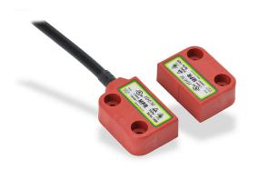
IDEM safety switch set, non-contact magnetic, right exit mount, (2) N.C. safety output(s), (1) N.O. monitoring output(s), plastic housing, 36 x 26mm, pigtail, 6.5ft/2m cable length.
