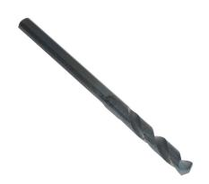
MK Morse pilot drill bit, replacement, 1/4in, split point, high-speed steel (HSS), bright finish, round shank, 5-5/16in overall length. For use with all MK Morse arbors.
